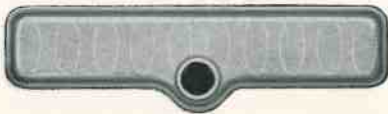
The above view shows the header end of the ceiling model. The dotted lines indicate tube positions.
