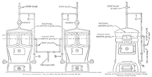
from one boiler to another in a multiple boiler system or from the boiler into the return pipe of the heating system.
