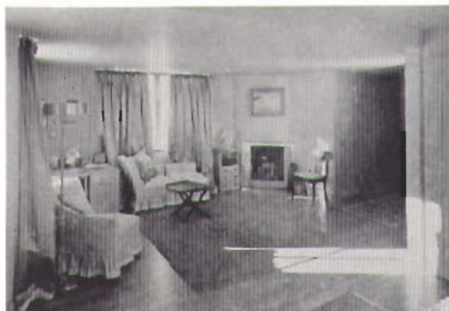
The master bedroom floor is comfortably tempered from the ceiling panel in the first story room directly below and with supplementary warmth, as required, provided by the ceiling panel in the bedroom.
