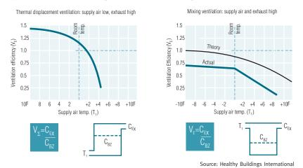
perspective, ventilation or "air-change" effectiveness is defined as the ratio of contaminant concentration in the return air to the contaminant concentration in the breathing zone of the room.
