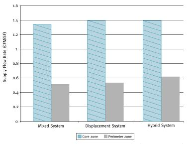
Comparison of Mixed, Displacement and Hybrid Underfloor System Flow Rates
