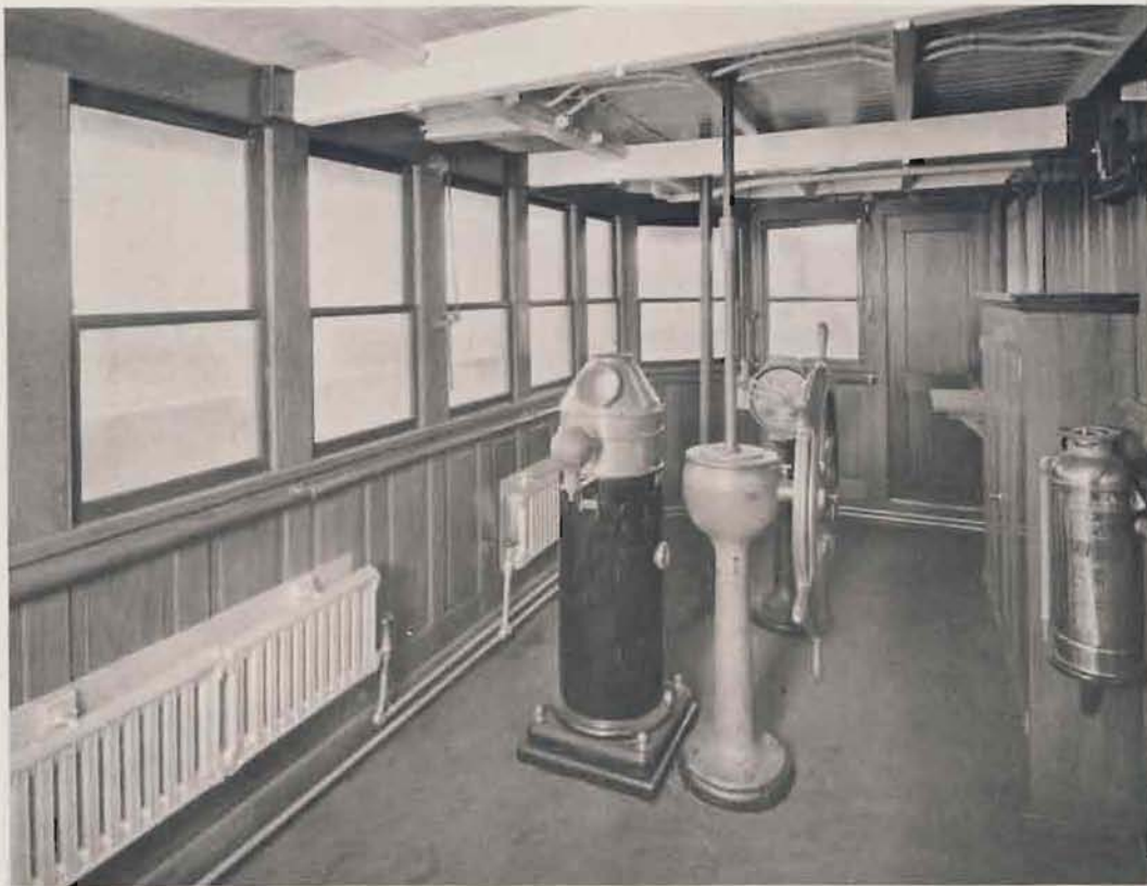
Many thousands of square feet of AMERICAN PEERLESS Wall Radiation were used in the vessels of the Emergency Fleet Corporation during the war. Picture shows AMERICAN PEERLESS Wall Radiators made of special non-magnetic material, used in over a hundred steamers built by the Submarine Boat Corporation at Port Newark, New Jersey.
