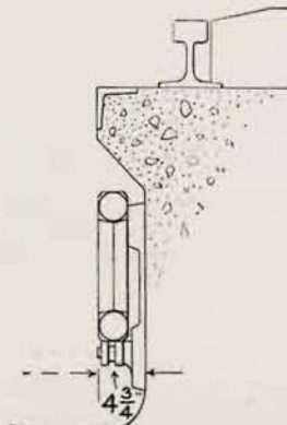
AMERICAN PEERLESS Wall Radiator recessed inside wall of engine pit.
