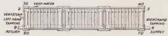
Fig. 511, 711 or 911. Assembled Three Sections in Single Tier— Water and One- and Two-Pipe Steam.
