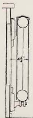
Detail of AMERICAN PEERLESS Wall Radiator supported by Arco Adjustable Wall Bracket.
