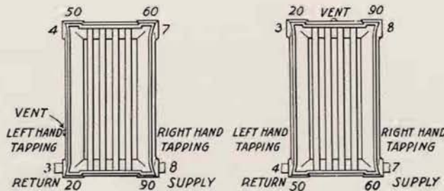
Fig. 54, 74 or 94. One- and Two-Pipe Steam.
