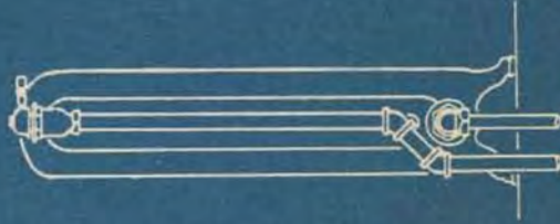
TWO METHODS OF CONNECTING RADIATORS FOR SUPPLY AND RETURN ON SAME END.
