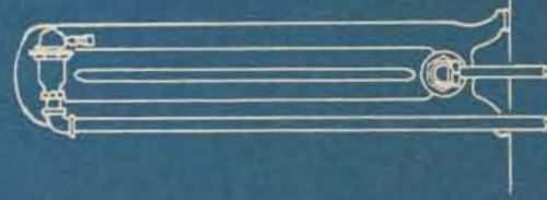
TWO METHODS OF CONNECTING RADIATORS FOR SUPPLY AND RETURN ON SAME END.
