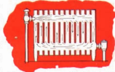
Fig. 3. Turbulence resulting from metering steam into radiators through jets at high velocity produces a close intermixture of steam and air right in the radiator and results in low radiator temperatures in mild weather. . . without resort to high vacuum. Individual control at the radiator is provided by the Webster Supply Valve. A Webster Radiator Trap keeps the radiator freed of condensation at all times.
