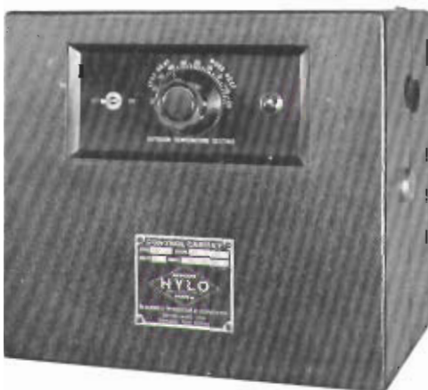
Fig. 16. Webster Type SP Hylo Variator Cabinet, approximately 12¼ in. wide, 11⅞ in. high, and 8¾ in. deep, may be located at a convenient operating point. Dial is adjusted when outdoor temperature changes and when more or less than normal heat is required. A switch gives remote shut-off. A lamp indicates that system is in operation. A schedule card (not illustrated) is placed on frame on top of cabinet. This frame adds 3½ in. to height of cabinet.
