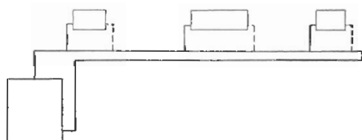
Fig. 46. Monoflo single main (one-pipe) hot water system.
