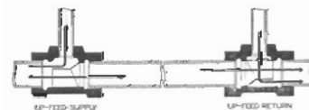
Fig. 174. Where structural characteristics of the installation might cause a question as to proper circulation, use both a Supply and Return Monoflo Fitting.
