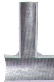
Shoulder prevents cross member from projecting into header.
