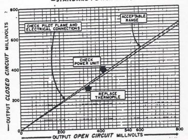
23 OHM POWER UNIT (CS434, CS591, CS5133, CS5134, CS5230, CS5278, CS5281, CS5296, VS8190, V8194, VS8233, VS8238, VS8262, VS8279, VS8291)
