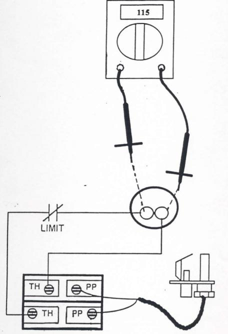
The reading taken directly across the thermostat is 115 millivolts. This reading added to the drop across the limit will be
