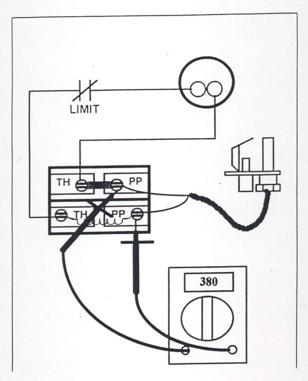
Closed Circuit with the controls in the circuit. This will measure the ability of the system to work with every resistance in the circuit.
