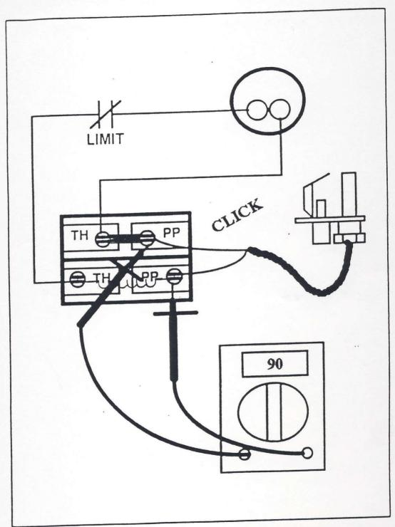
Drop out is done by blowing out the pilot and waiting for an audible click or a slight jump in the meter needle. An other way to check this is to shut off the flow of gas to the pilot and have the main burner running. When the main burner goes out that is the drop out.
