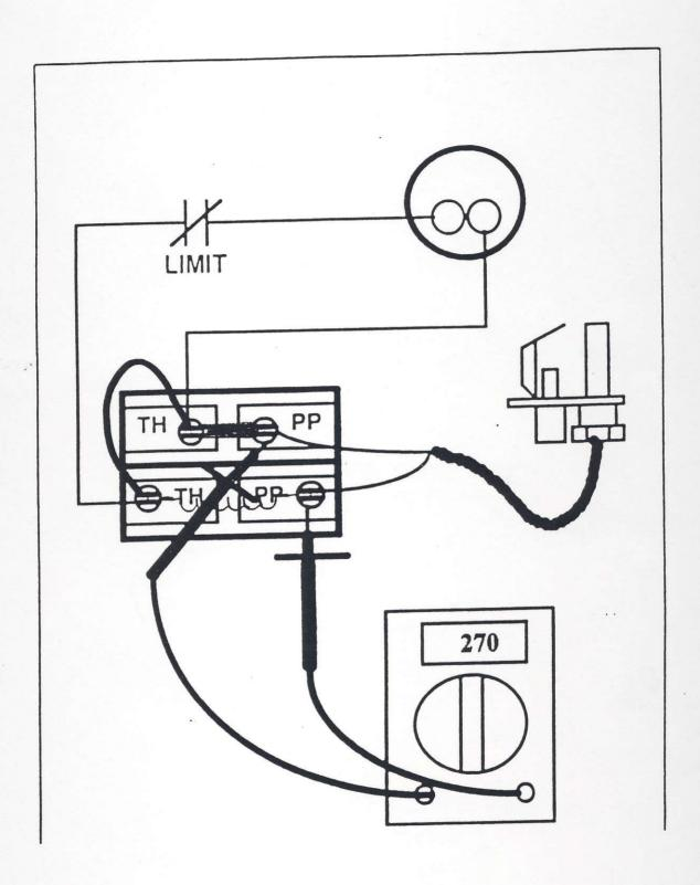
Closed Circuit with the controls "Jumped Out". This will measure the voltage drop across just the coil in the valve.
