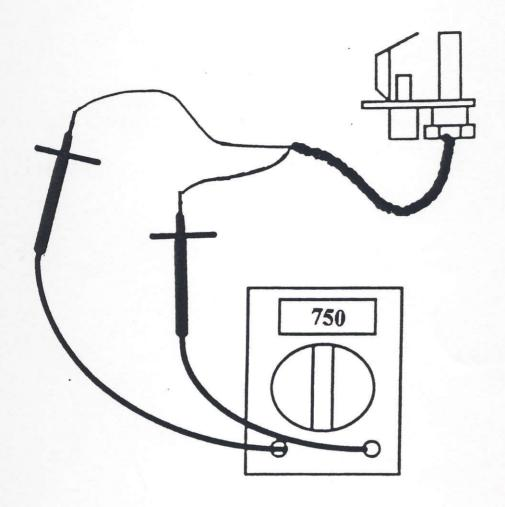
Open Circuit minimum 540 millivolts. It is taken with the generator disconnected from the valve.
