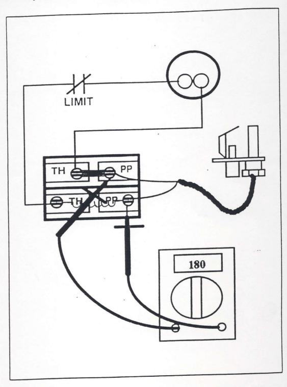
The pull in with the controls jumped out is usually taken when the valve will not open with the controls in the circuit, or when the pull in with controls in the circuit is high. It will help you to see if the problem is in the controls or valve coil. This reading should be between 95 to 179. A high reading would indicate a bad valve coil.
