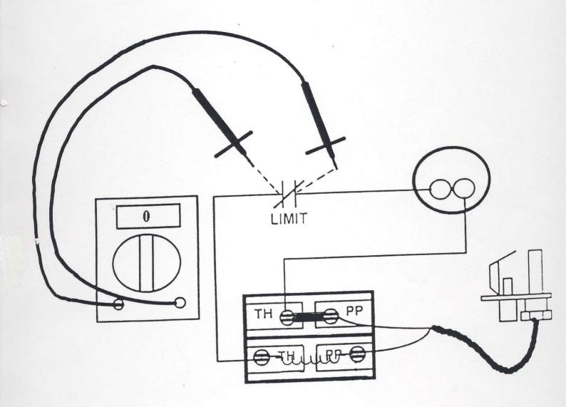
Limit is 0 to 10 millivolts and is the same for any switch.
