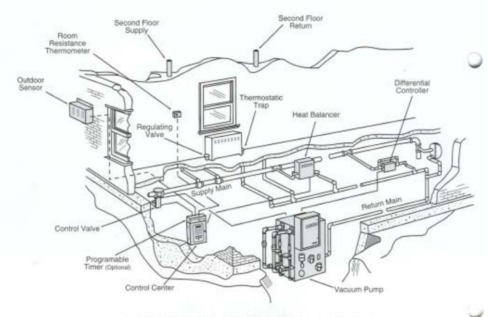
MEPCO's Vari-Vac Differential Steam Heating System creates energy-efficient heating while employing a building's original pipes and mains. See back cover for the descriptions and functions of the system's component parts.
